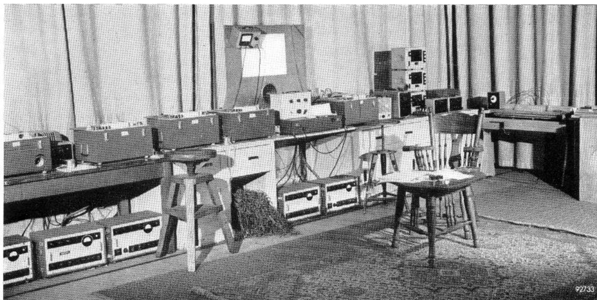
Fig. 1. Part of the equipment employed in the Philips Research Laboratories for making the electronic ballet music "Cain and Abel". On the table are some of the seven magnetic tape recorders used (sometimes five at a time). Also to be seen are a number of amplifiers, a mixing desk, filters, metronomes, various electronic sound-sources, loud-speakers, etc.
